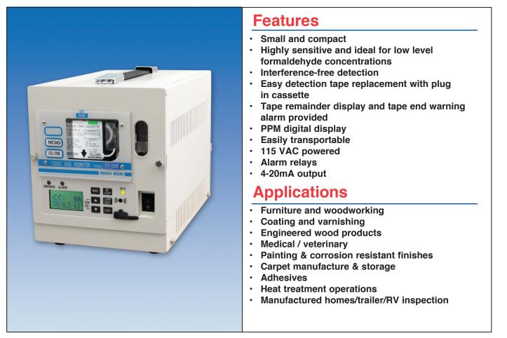
RKI's paper tape monitors utilize highly sensitive colorimetric tapes to achieve interference free gas detection. The FP-330 is equipped with an easily replaceable tape that is highly specific to Formaldehyde. This model is equipped with a digital display showing the type of gas and concentration in PPM. The FP-330 will also display remaining tape life as well as an end of tape alarm.
